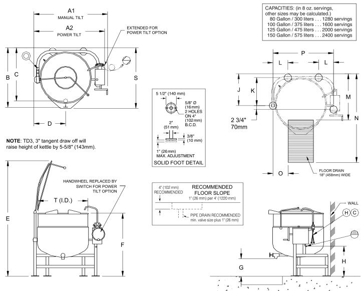
UNIT SHOWN WITH OPTIONAL 2" TANGENT DRAW-OFF VALVE, SPRING ASSIST COVER, HOT AND COLD WATER FAUCET AND STEAM CONTROL KIT.
